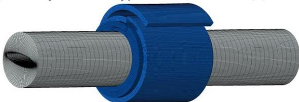
Figure 1: Cuff model (in blue), designed by thickness of 2 mm and length of 17 mm, in interaction with the urethral model (in grey).
