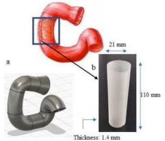
*Figure 1: Comparison between physiological duodenum and a) anatomical technical drawings. b) PDMS prototype.*
