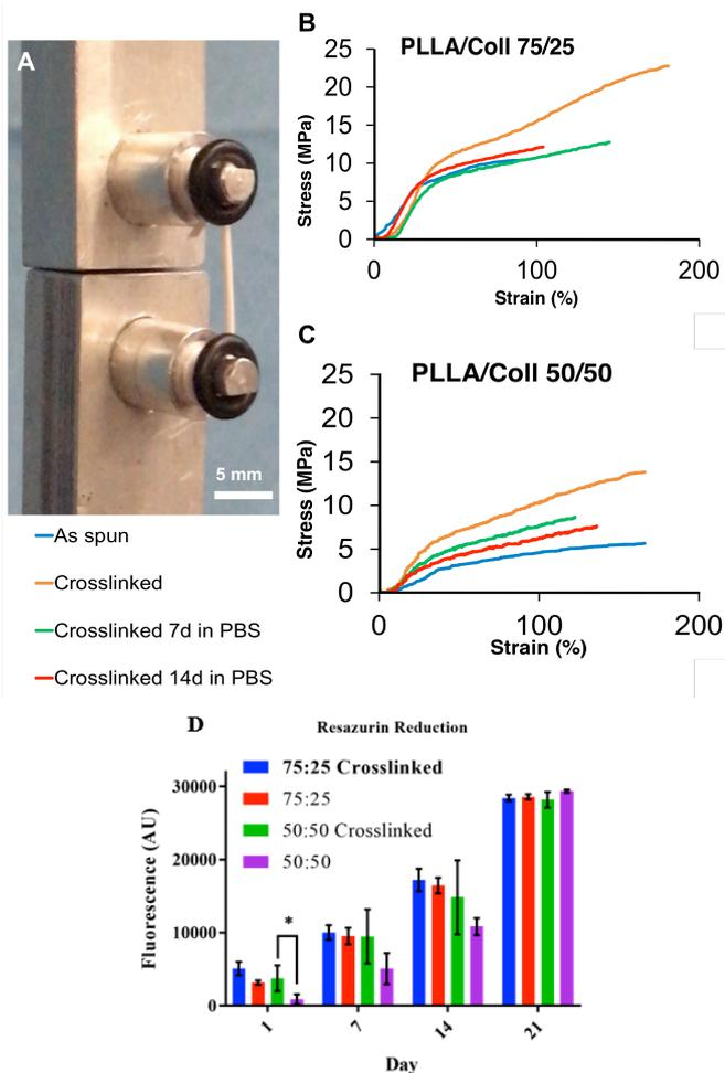
Fig.2: A) Capstan grips with a bundle; B) Stress-strain curves for PLLA/Coll 75/25; C) Stress-strain curves for PLLA/Coll 50/50. D) Cell viability of NTF-322 on bundles.
