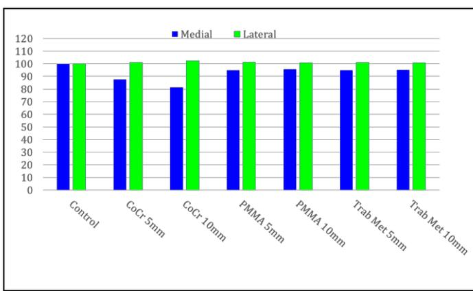
Figure 1: medial and lateral average bone stress in the control and for the different materials and thickness in the case of femoral augment
