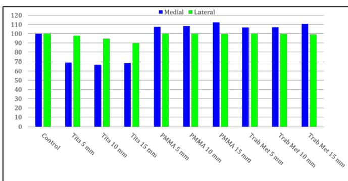
Figure 1: medial and lateral average bone stress in the control and for the different materials and thickness in the case of tibial augment
