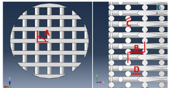
Figure 1. Geometrical input parameters of the scaffold: layer orientation (A), offset (B), fibre diameter (C) and pore size (D).
